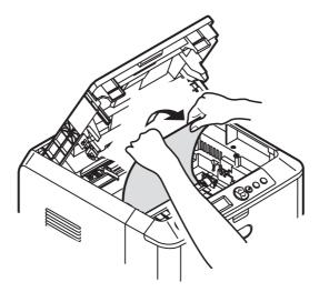
**5.** Re-install the image drum complete with toner cartridge, ensuring that the pegs (1 & 2) correctly locate into the slots on each side of the printer (3).
